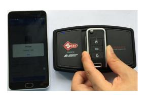
Press any button of the remote, when "creating 100%" comes out, the remote is generated.
