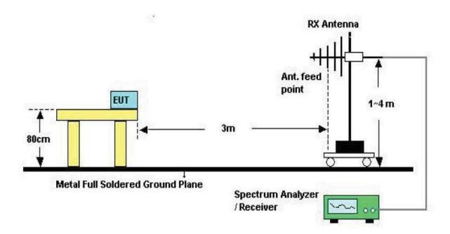
Above 30MHz Test Setup
