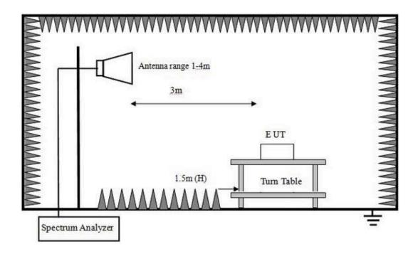
Above 1GHz Test Setup
