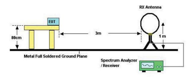
Below 30MHz Test Setup
