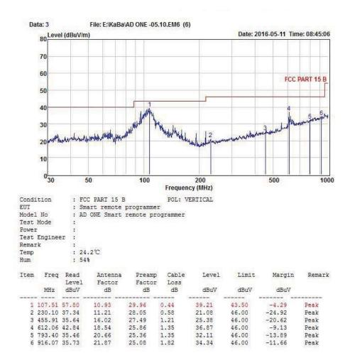
Remark: Level = Read Level + Antenna Factor - Preamp Factor + Cable Loss
