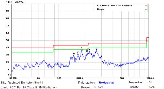
Limit: FCC Part15 Class B 3M Radiation Mode:TX 2480
