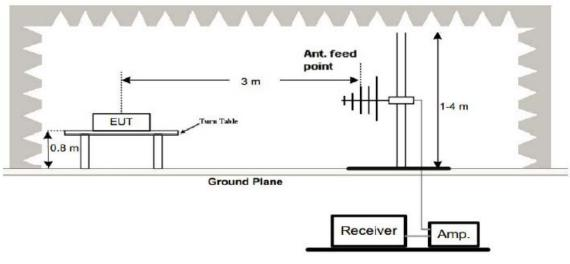
(3) Radiated Emission Test-Up Frequency Above 1GHz
