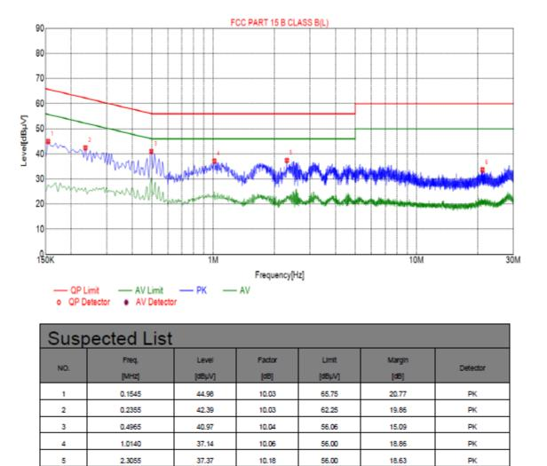
Remark: Transd = Cable lose + Antenna factor - Pre-amplifier; Margin = Limit – Level
