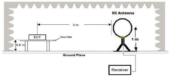
(2) Radiated Emission Test-Up Frequency 30MHz~1GHz
