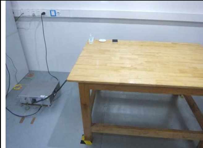
Conducted Emissions Test Setup Front View
