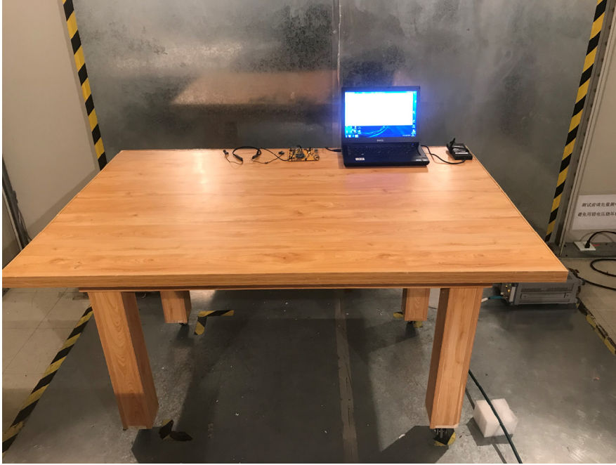
Conducted Emissions (Side View)
