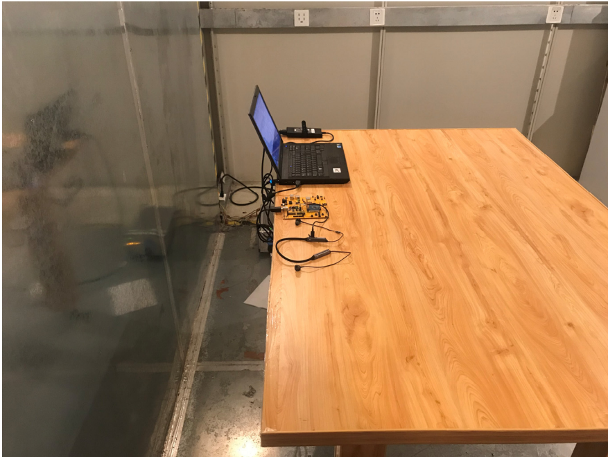
Conducted Emissions (Side View)
