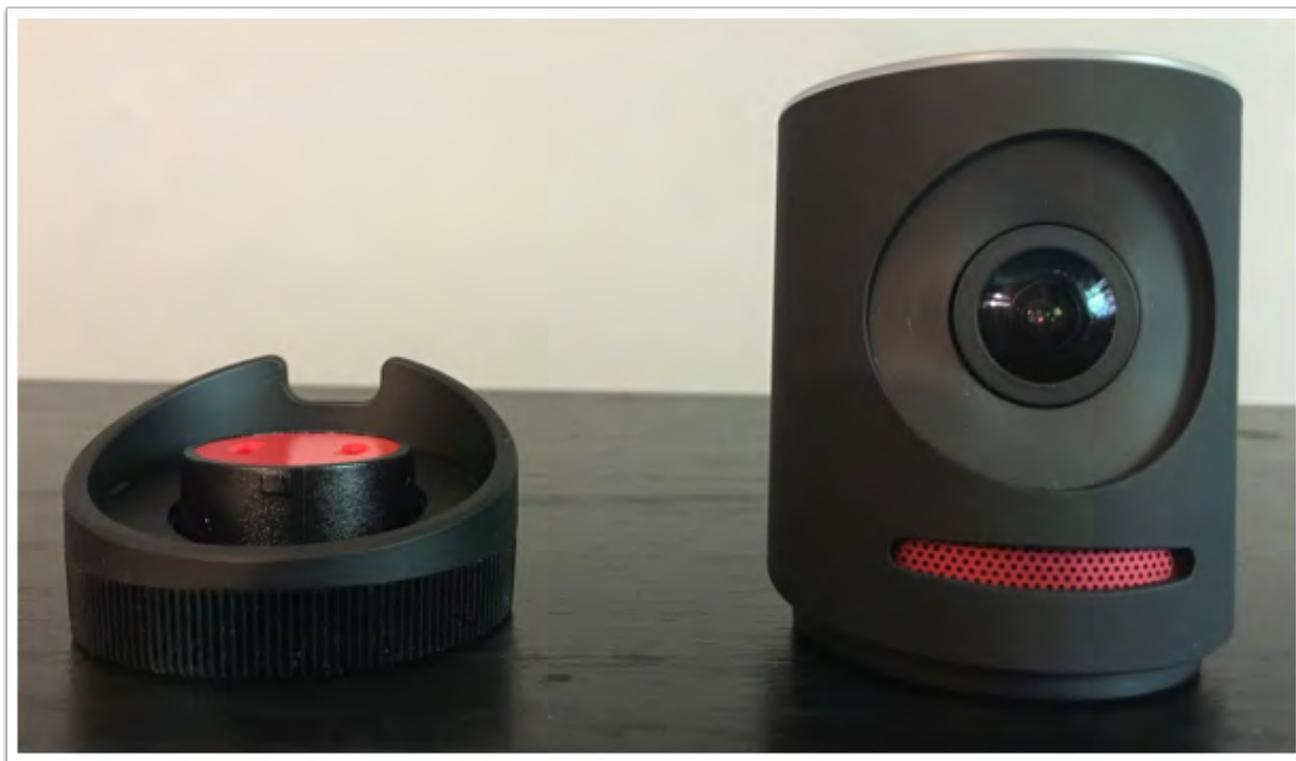
Place the Mevo on top of it. The micro-USB port on the back of the Mevo should match up with the opening for the Micro-USB cable on the back of the mount
