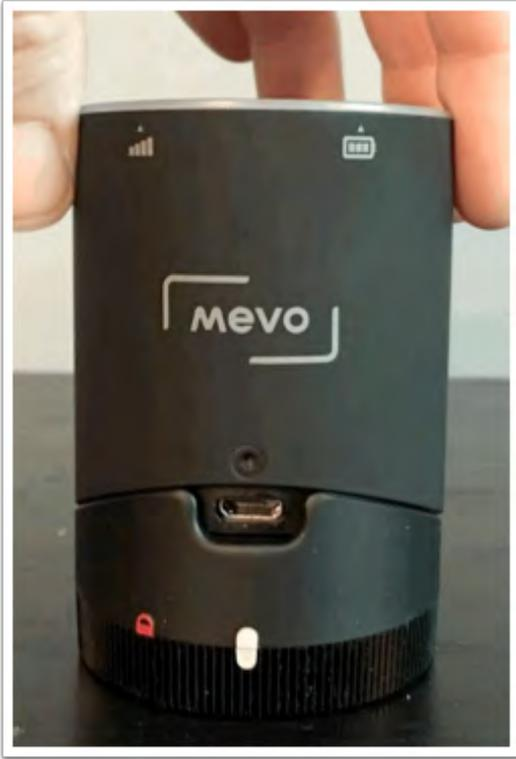
On the back of the mount, you should notice two white tabs, with a red padlock icon to the left. Turn the twist-lock ring so that the bottom white tab lines up with the red lock.
