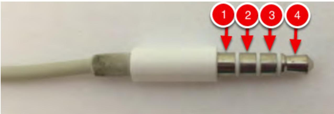
The red arrows above are pointing to three chrome rings and a chrome tip separated by three much thinner rings. This is referred to as a TRRS plug (tip-ring-ring-sleeve). This is the correct type of audio input that iOS devices can accept.
