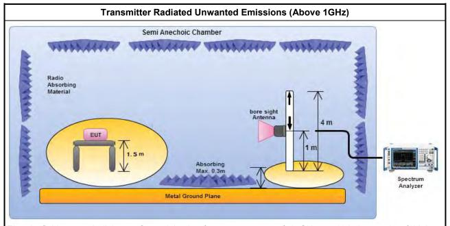
Electric field tests shall be performed in the frequency range of 1 GHz to 10th harmonic of highest fundamental frequency or 40 GHz using a calibrated horn antenna.
