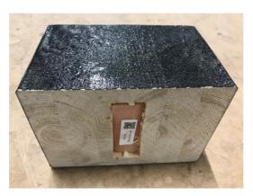
Figure 4. The mounting position of the Pallet tracker inside the middle block of the pallet.
