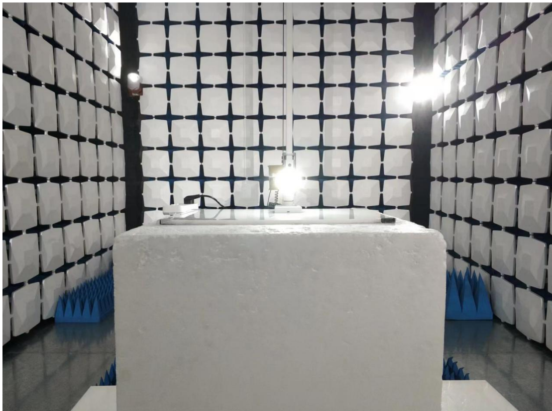
Above 1GHz for radiated emission test setup
