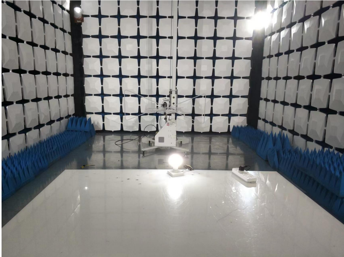
Blow 1GHz for radiated emission test setup
