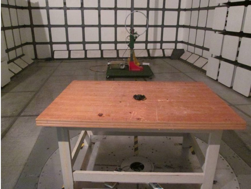
Radiated Emissions View (Below 30 MHz)
