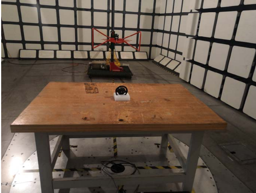
Radiated Emissions View
