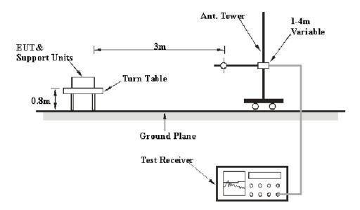
The radiated emission tests were performed in the 3 meters, using the setup accordance with the ANSI ANSI C63.10-2013. The specification used was the FCC Part 15.235(a) & 15.235 (b) &15.209 limits.
