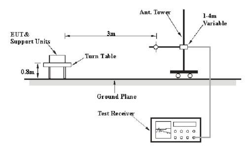
The radiated emission tests were performed in the 3 meters, using the setup accordance with the ANSI C63.10-2013. The specification used was the FCC Part 15.235(a) & 15.235 (b) &15.209 limits.
