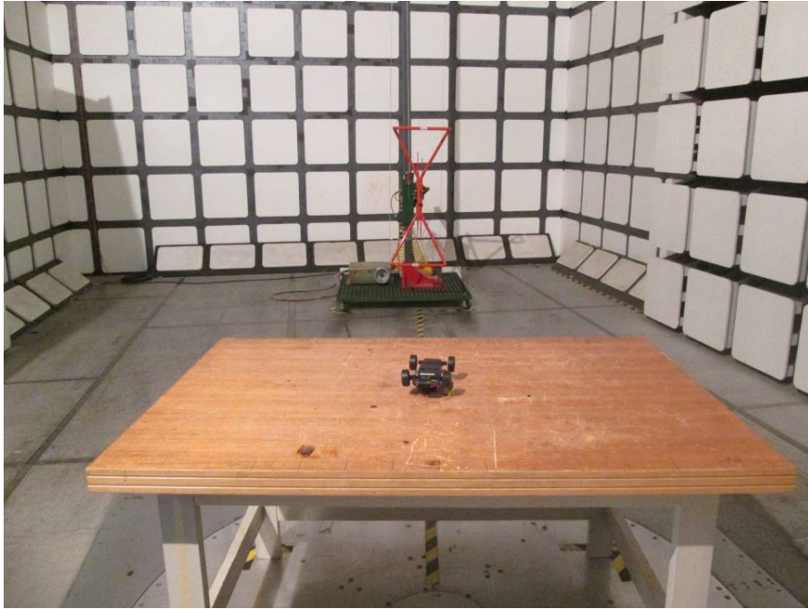
Radiated Emissions –Front View
