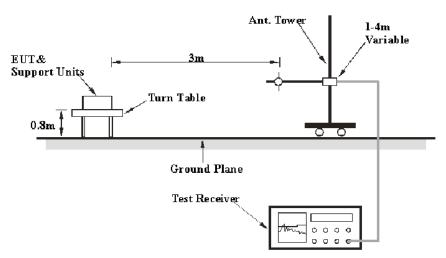
The radiated emissions were performed in the 3 meters distance, using the setup accordance with the ANSI C63.10-2013. The specification used was the FCC Part 15.209 and FCC Part 15.229(a) & 15.229 (b) limits.
