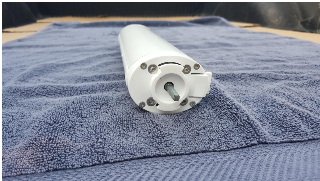
Figure 1. Top of EUT with Motor Shaft Exposed
