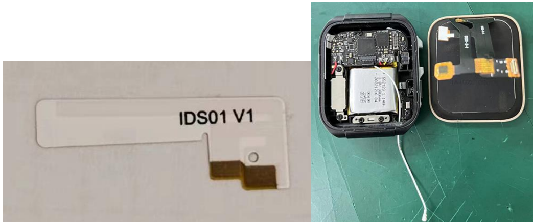
Figure antenna structure
