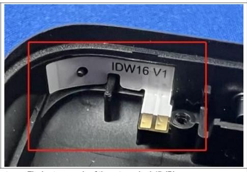
The antenna is FPC antenna. The best case gain of the antenna is -1.47 dBi.
