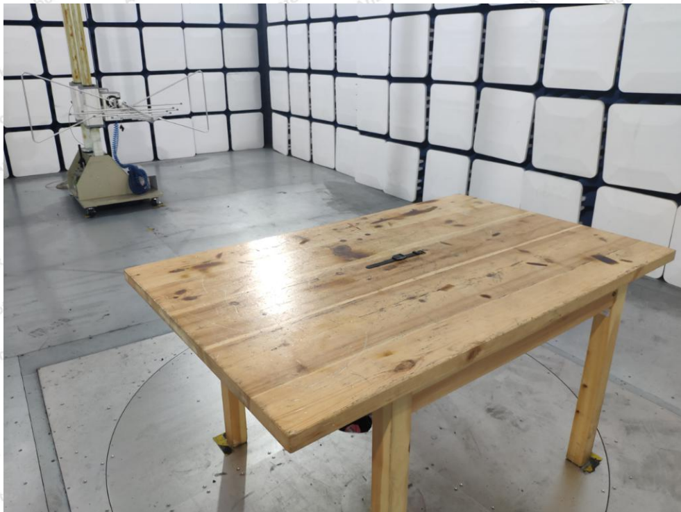
Photo of Radiation Emission Test
