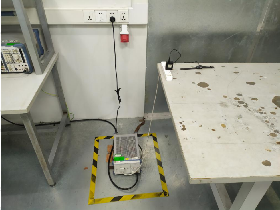
Photo of Conducted Emission Measurement
