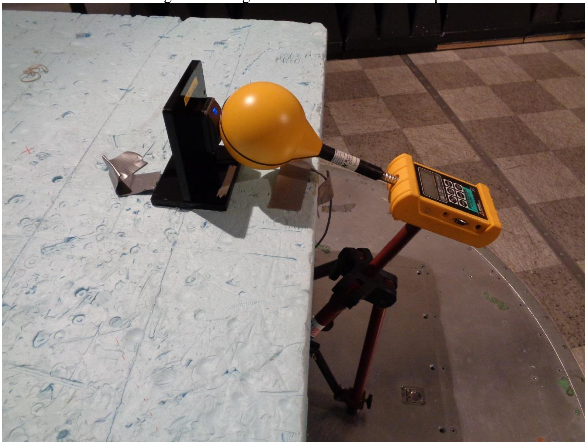
Figure 5 – Magnetic field measurement setup
