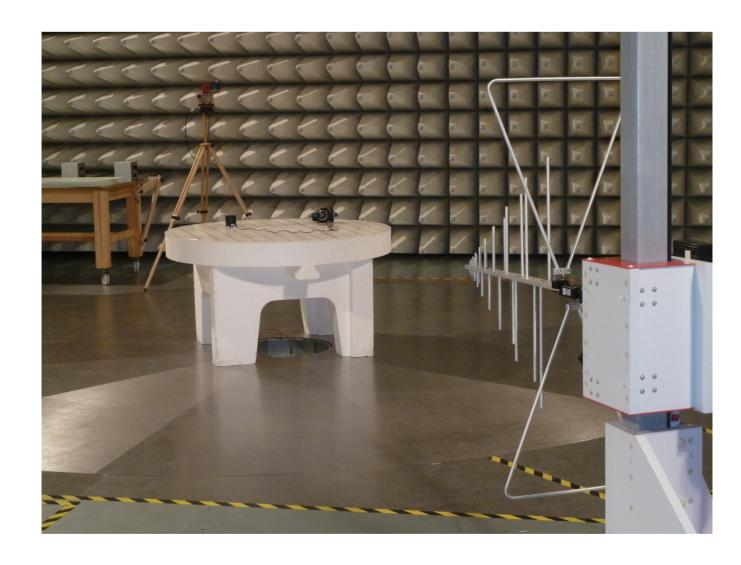
Description: Test setup emissions up to 1 GHz – USB
