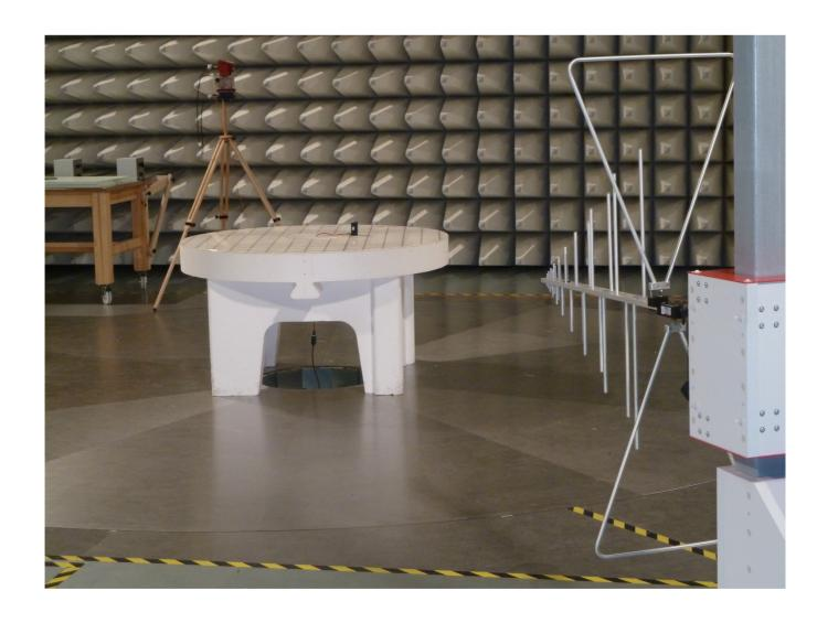
Description: Test setup emissions above 1 GHz – Bluetooth + Audio mode
