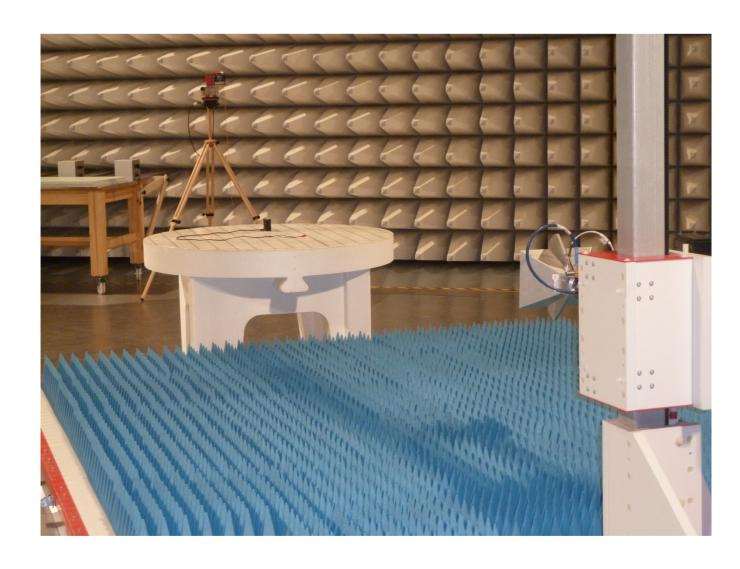
Description: Test setup emissions above 1 GHz – USB mode
