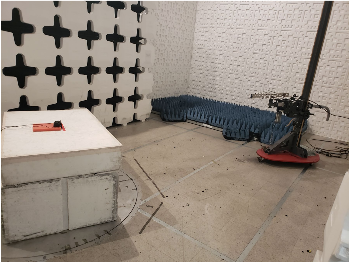
Figure 4. Radiated Emissions Test Setup, 200 MHz to 1GHz
