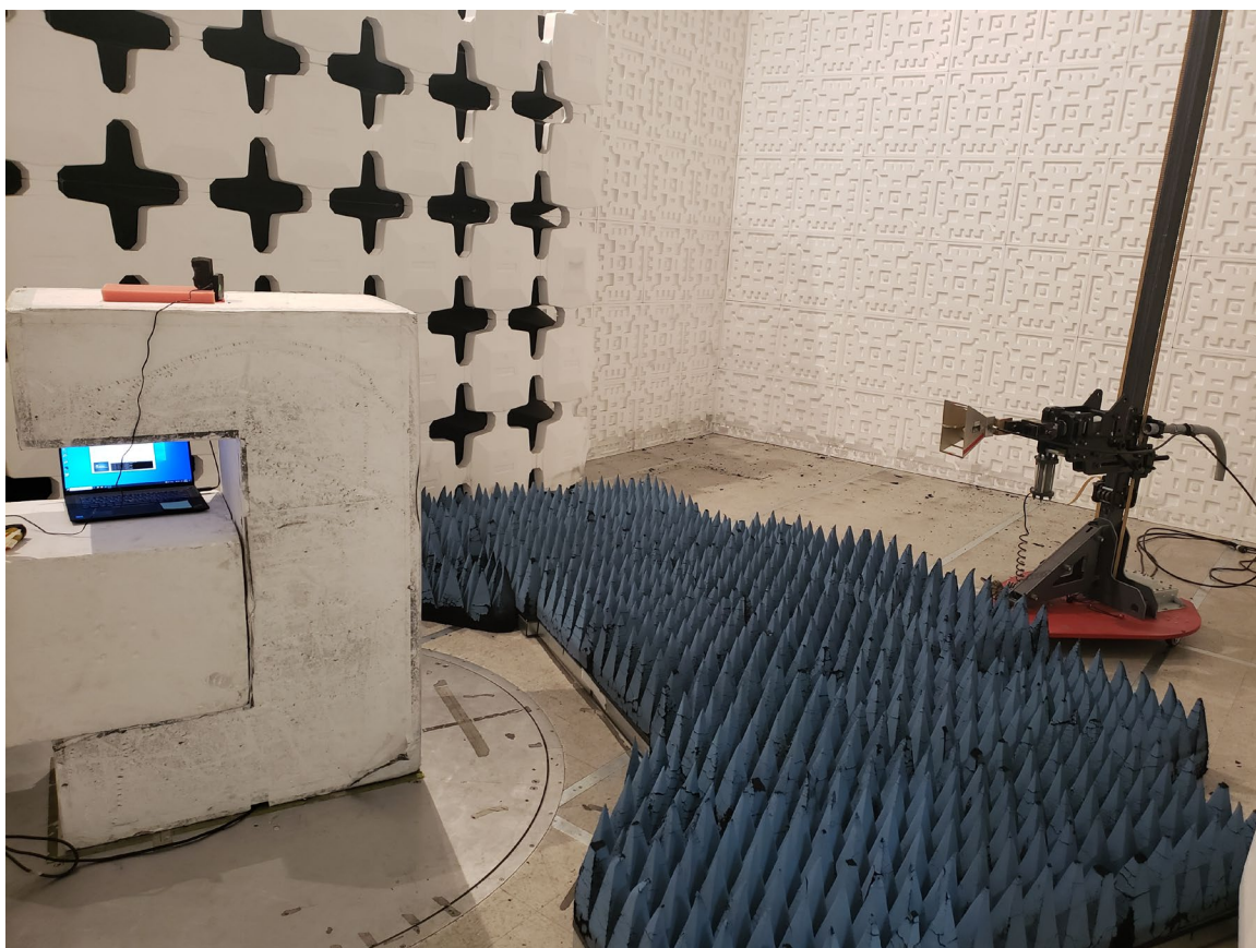
Figure 5. Radiated Emission Test Setup, above 1 GHz
