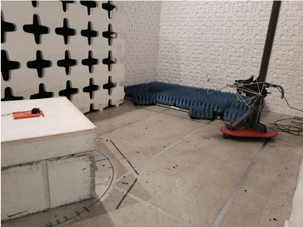
Figure 3. Radiated Emissions Test Setup, 30 MHz to 200 MHz, Back
