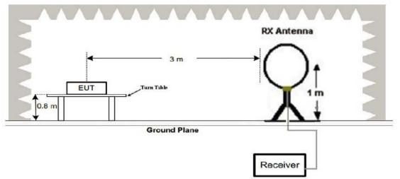
(2) Radiated Emission Test-Up Frequency 30MHz~1GHz
