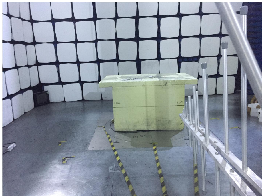
Radiation Emission Test Setup (30MHz to 1GHz)
