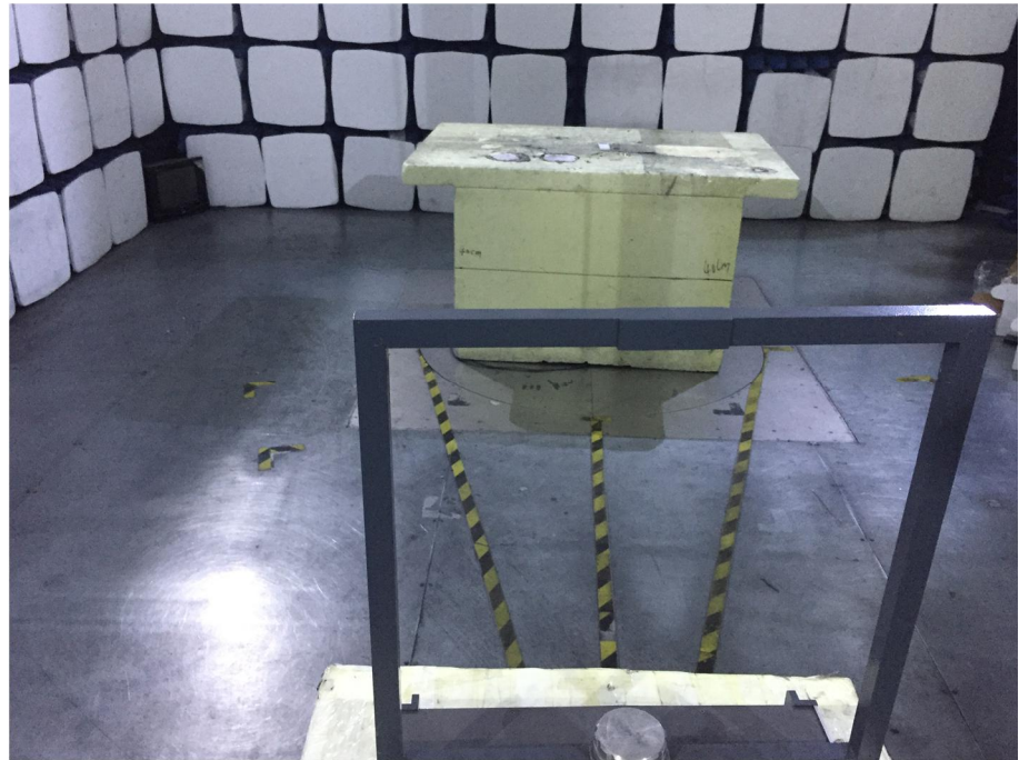
Radiation Emission Test Setup (Below 30MHz)
