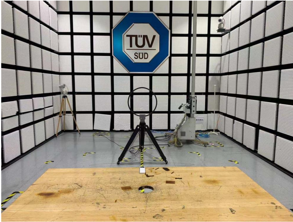
Radiated Emission Setup 9kHz ~ 30MHz
