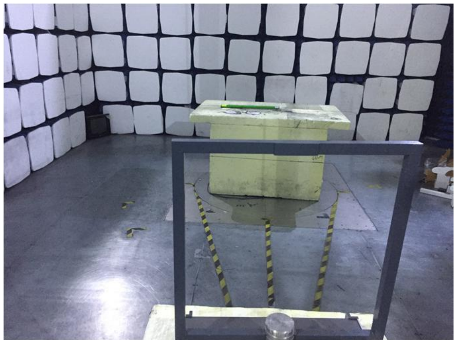
Radiation Emission Test Setup (Below 30MHz)
