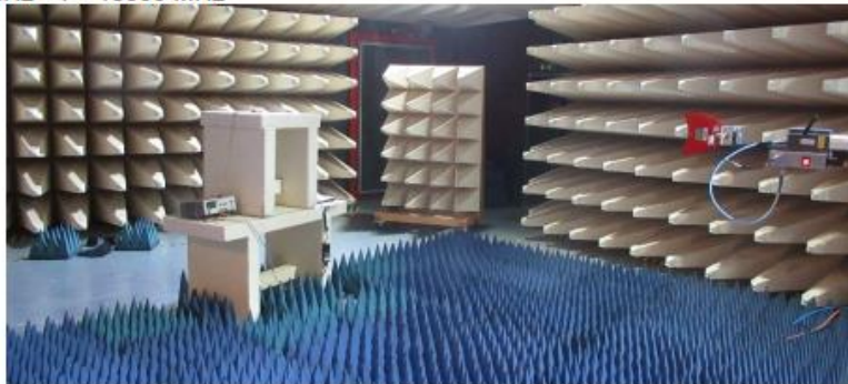
Anechoic chamber Test Setup 1000 MHz < f < 18000 MHz
