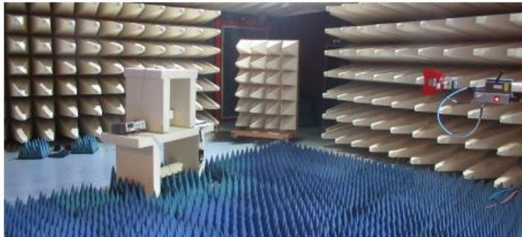
Test Setup 1000 MHz < f < 18000 MHz
