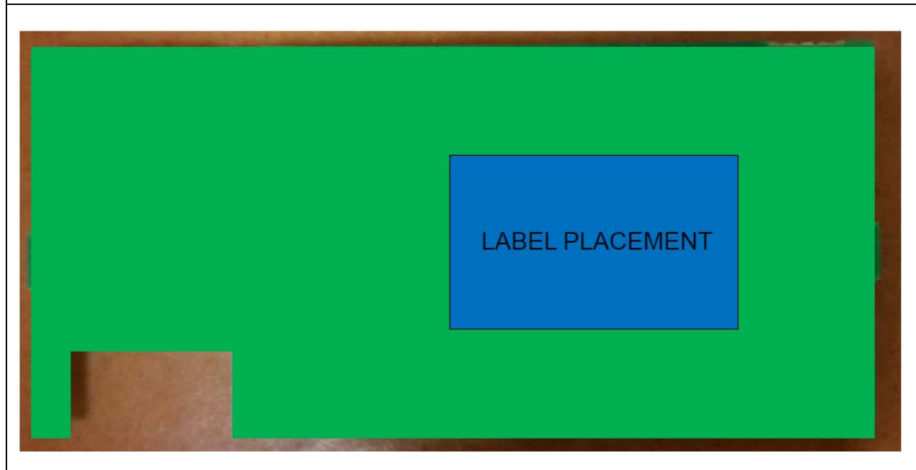
Module Label Placement (Bottom of PCB)
