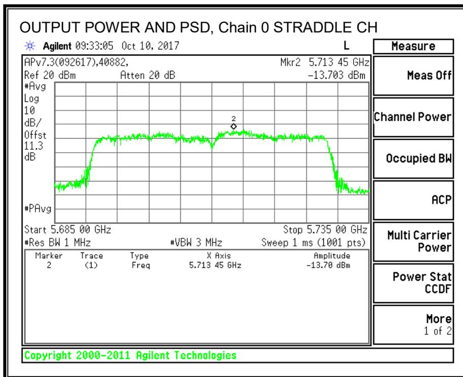
Note – Straddle channel tested to 5.6 GHz band settings as this is considered worst-case.
