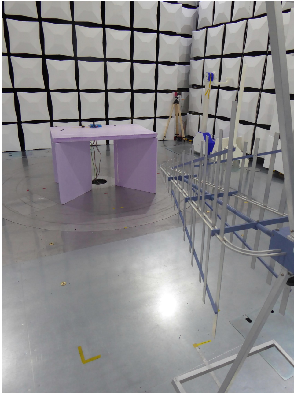
Test setup semi anechoic chamber M276, 30 MHz – 1 GHz
