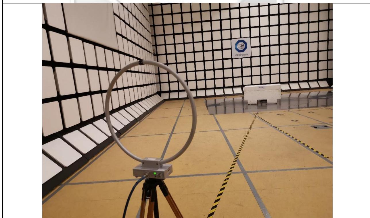
Radiated Emissions (Spurious Emissions Inclusive Restricted Bands Requirement) Test Setup (Rear View)
