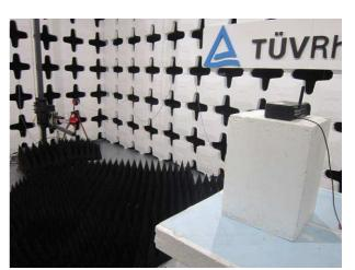
RADIATED TEST SETUP
