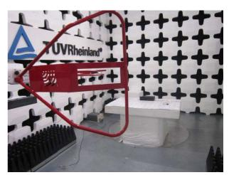
RADIATED TEST SETUP
