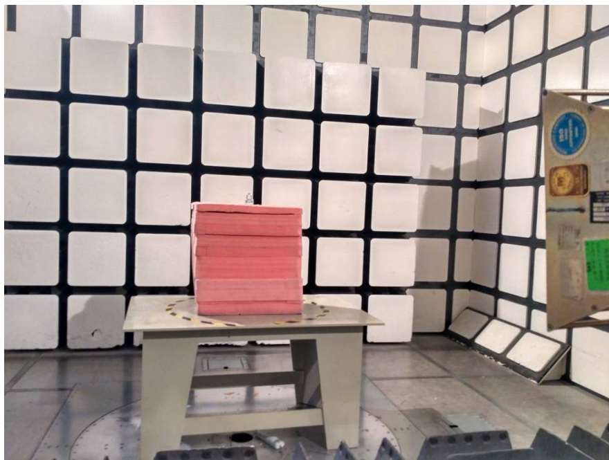
Radiated Emissions View (Above 1 GHz)
