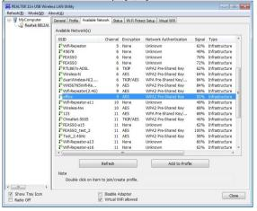
3. If the wireless network uses encryption, you need to input the correct encryption key. The configuration utility automatically suggests the correct authentication type (see the drop-down list), and you should not change the suggested value.
