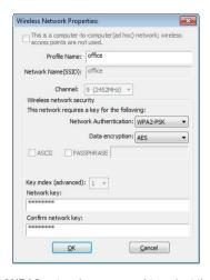
**NOTE:** For WPA/WPA2 networks, you need to select the correct encryption type, as well (AES or TKIP). These settings depend on how the wireless network is set up. Only the owner of the wireless network can provide the required information.
