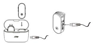
To charge, plug your charging case or microphone into a power source using the included USB Type-C cable.
