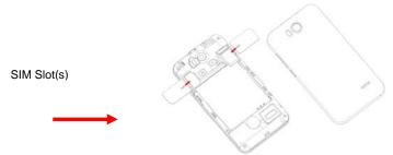
3. Replace the rear cover of the mobile phone and power on.
