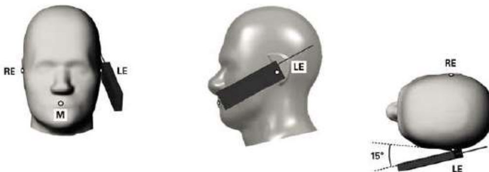
Fig.11.4 Illustration for Tilted Position
