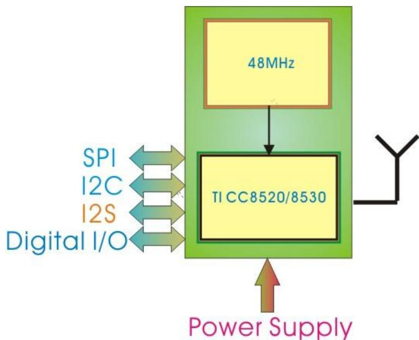
**Note: I2C must be connected to external pull-up resistor  $2.7\text{K}\Omega$  . VBAT has internal resistor  $100\text{K}\Omega$  on Module.**
