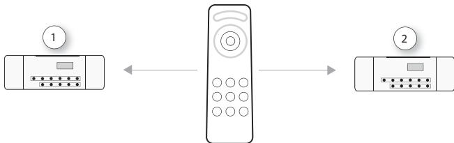
Note: Each zone can handle 1 Parent Controller and up to 10 Child Receivers.
