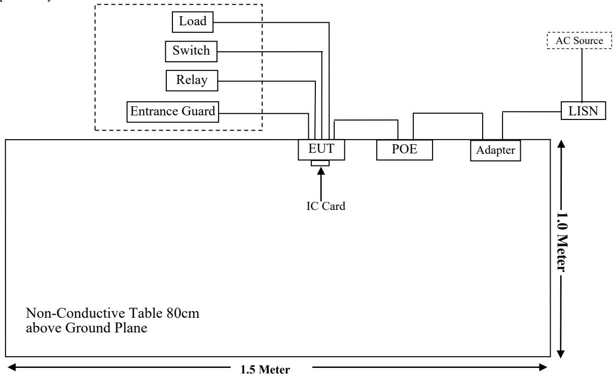
For Radiated Emissions (Below 30 MHz & Above 30 MHz):
