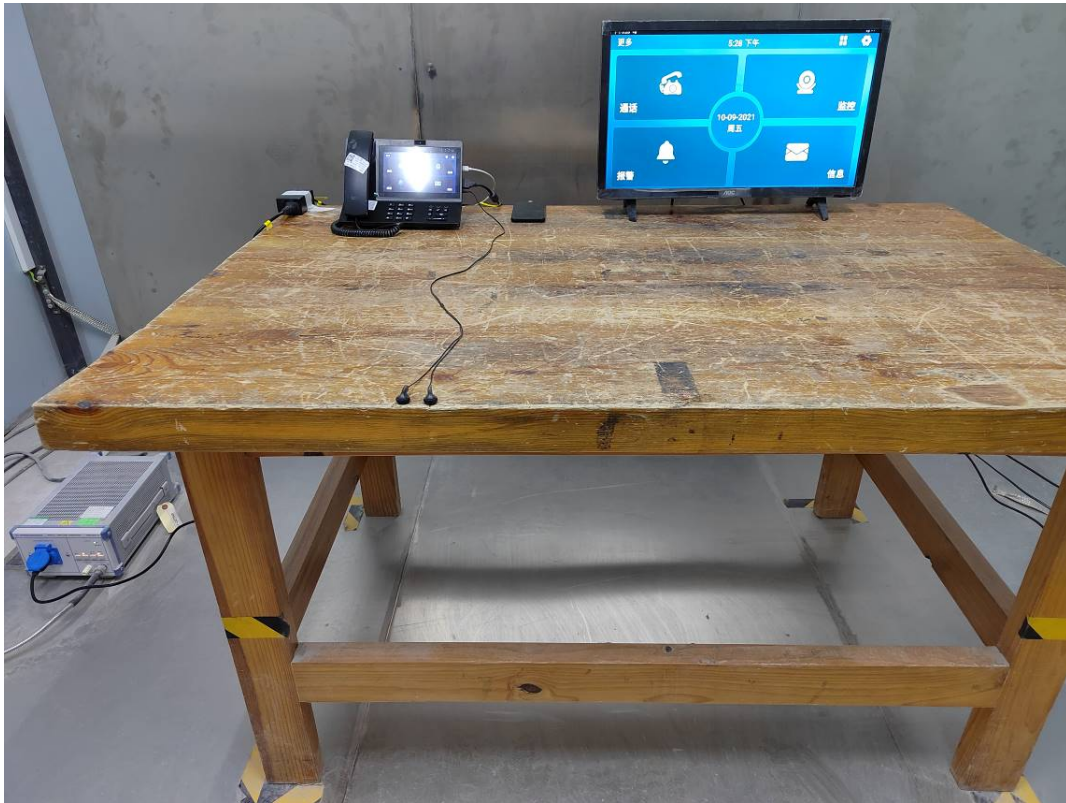
Conducted Emissions Side View- POE
