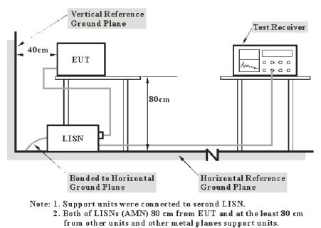
The setup of EUT is according with per ANSI C63.10-2013 measurement procedure. The specification
