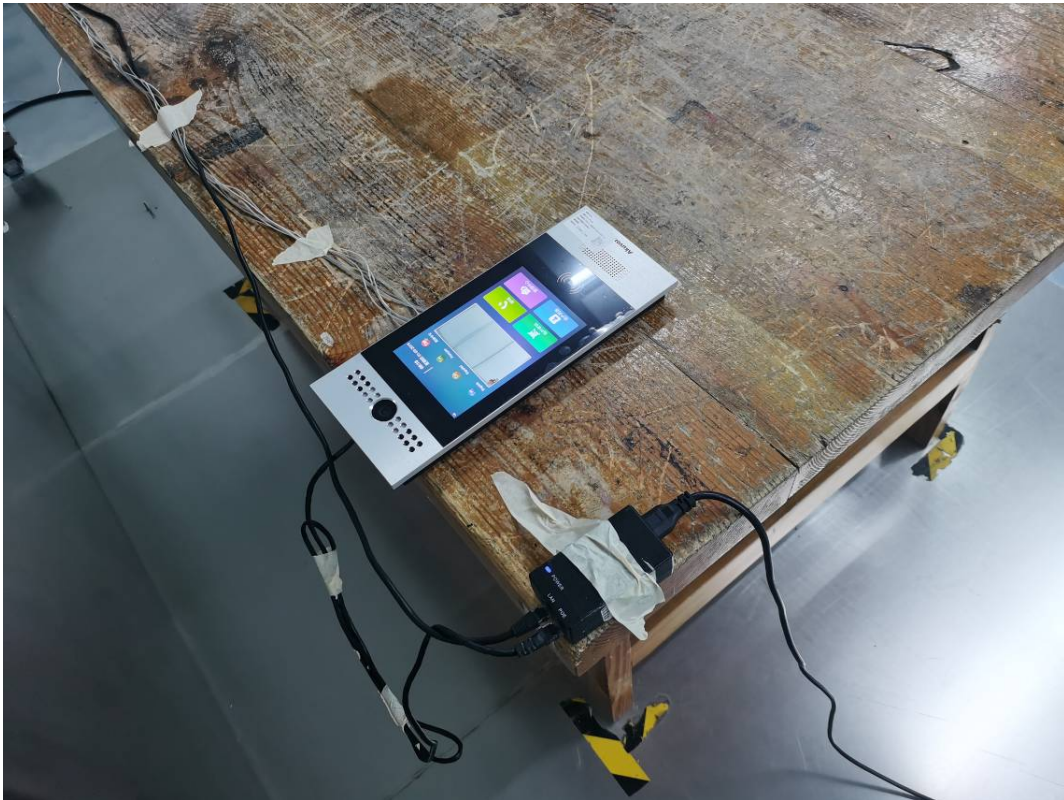
Conducted Emissions Side View-Powered by POE
