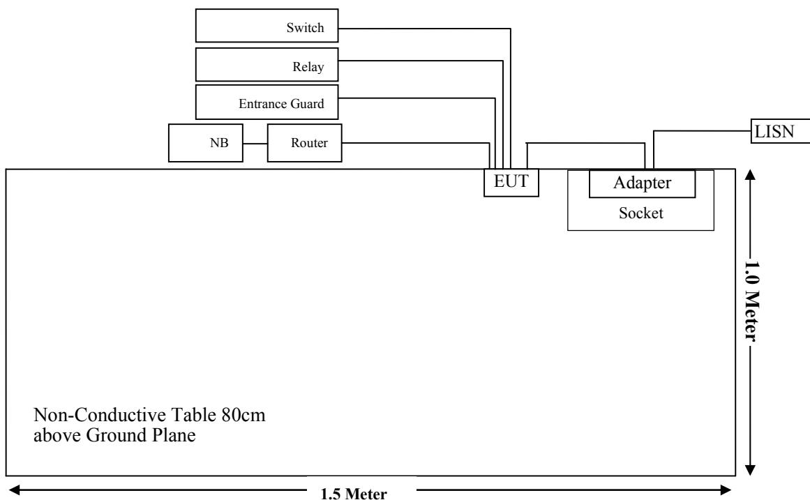
For Radiated Emissions (Below 1GHz&Above 1GHz):
