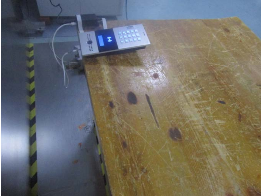
Conducted Emissions – Side View(POE)
