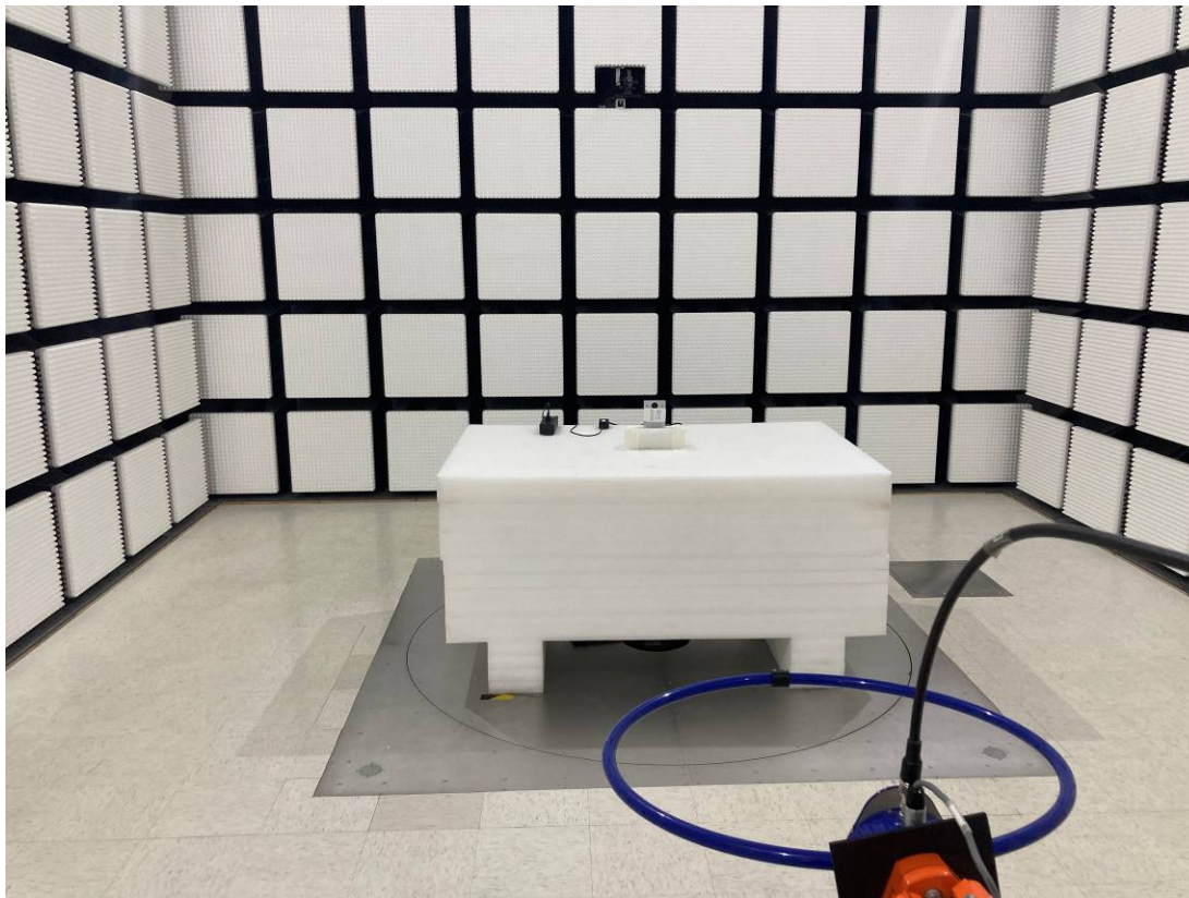
Radiated Emission 30M-1GHz View POE
