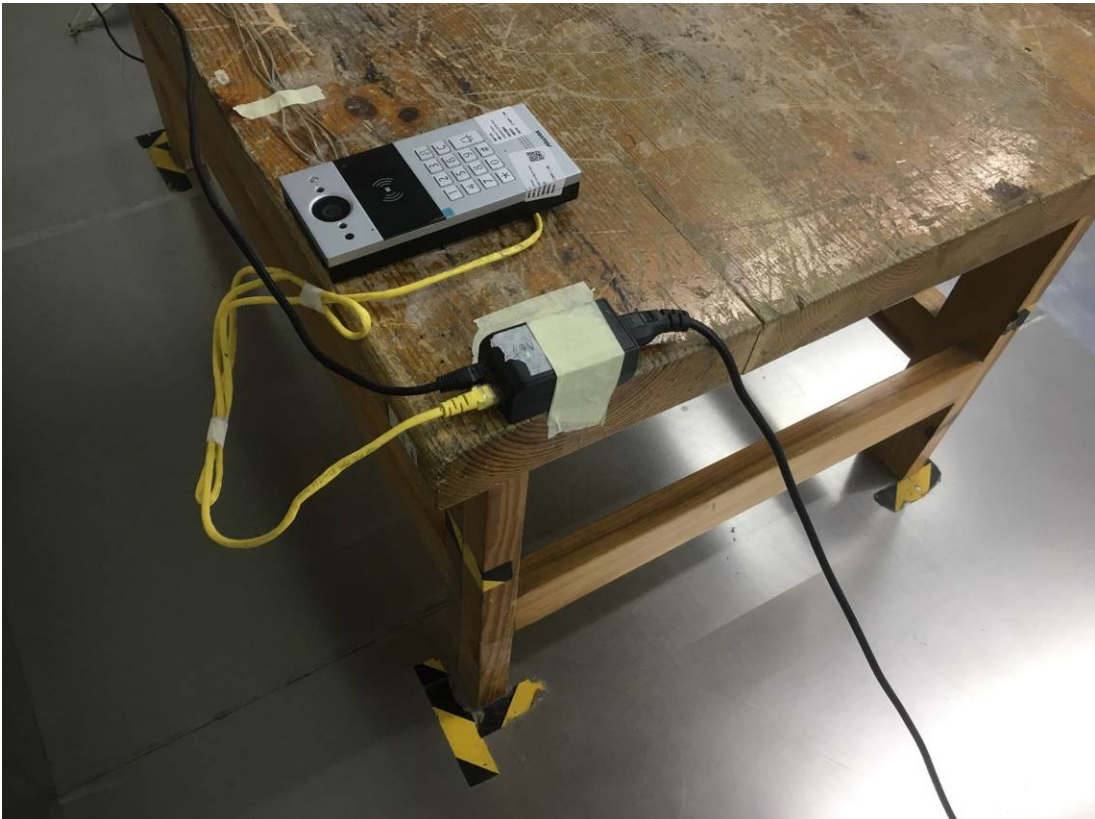
Conducted Emissions Side View POE
