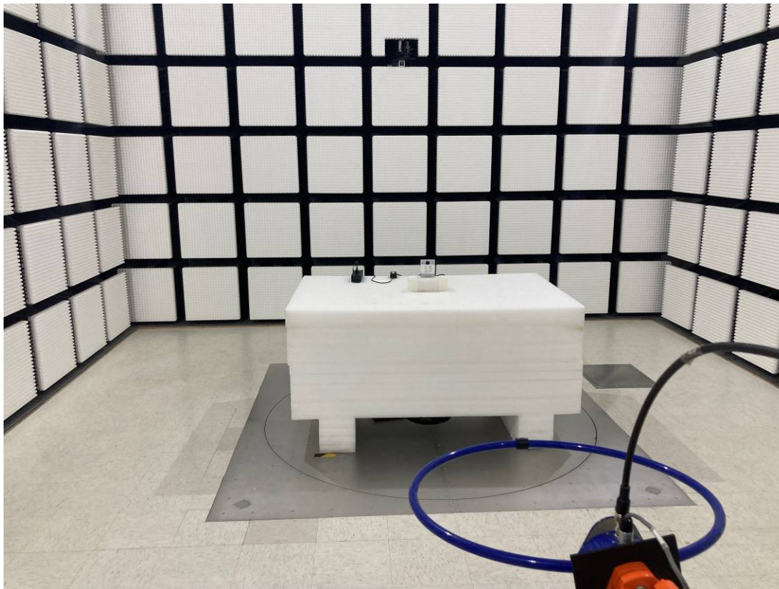
Radiated Emission Below 1GHz View POE
